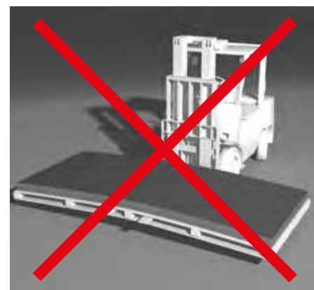
Improper forklift transport
